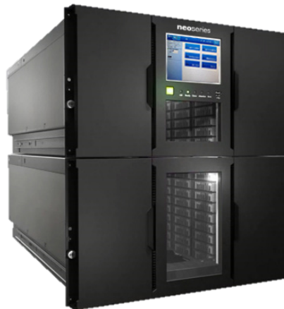
The NEOxl 80 Tape Library consists of a basic module with 80 cartridge slots and 6 tape drives with scalability to 560 slots and 42 tape drives with expansion modules.
