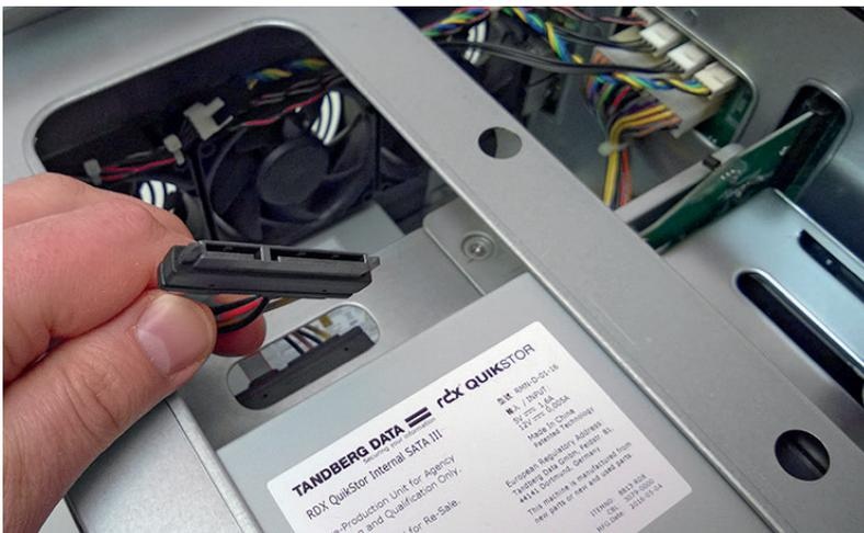
Inside, the NAS is already set up for direct connection, via a single Serial ATA and power cable. ***This can therefore be carried out by any IT technician with a minimum of experience and takes no more than 5 minutes.***
