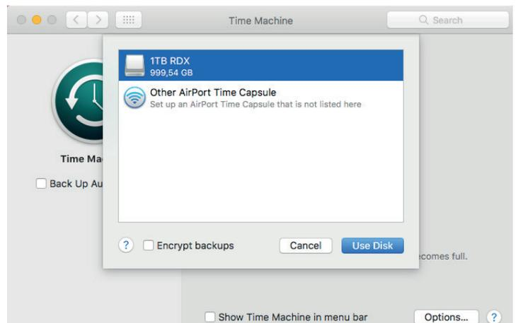
After that, Time Machine is set up and ready to perform its first backup. We recommend checking the box “Back Up Automatically”. If done, the first backup starts after 120 seconds. Further backups will then be performed every hour. We advise implementing media rotation with at least three media for full disaster protection with off-site storage. Therefore, further RDX media can be easily introduced to Time Machine. Media should be alternated on a daily basis.
