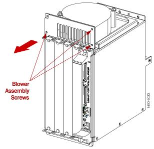
Figure 2. Blower Assembly Attachment Points
