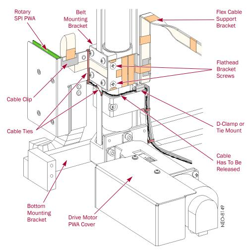
Figure 3-1: Base of Rear BDA and Connected Components
