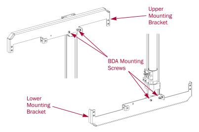
Figure 2-4: UHA and LHA Mounting Screws
