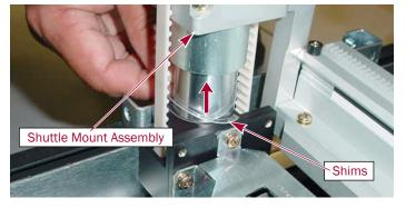
Figure 3-7: Slide Shims up the BDA
