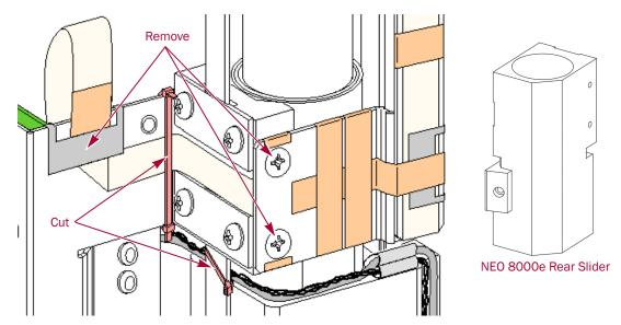
Figure 3-4: Clip, Cable Ties, and Screws to be Removed
