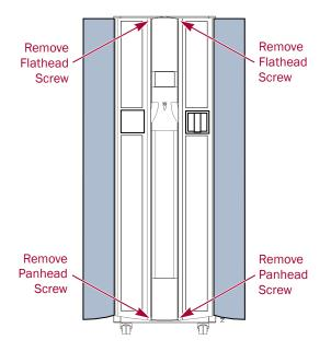
Figure 1-6: Front Panel Assembly Screw Locations
