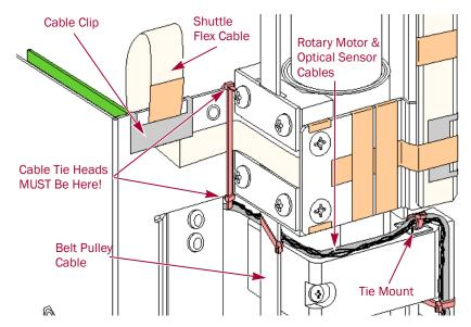
Figure 3-19: Securing the Cables with New Cable Ties
