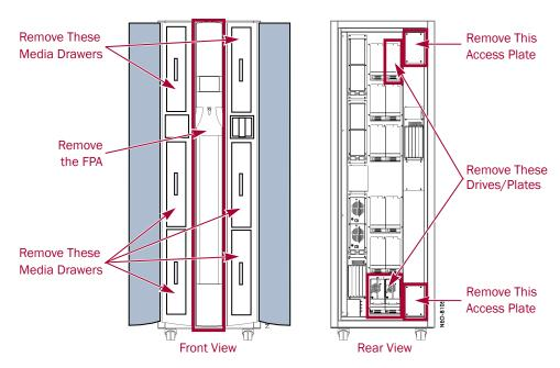
Figure 1-2: Access Plates and Components That Need To Be Removed
