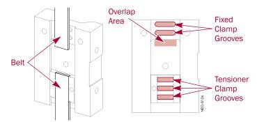
Figure 2-8: Belt Backplate Showing Clamp Grooves
