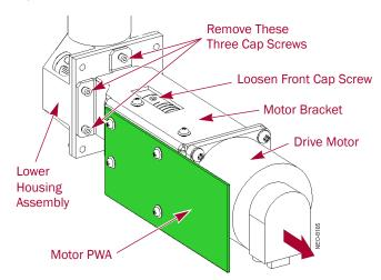
Figure 3-11: Location of the Drive Motor Screws
