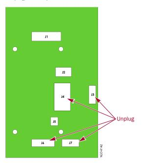
Figure 3-3: Location of the Rotary SPI PWA Connectors
