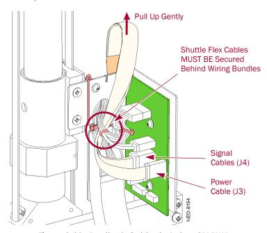
Figure 3-20: Reattach Cables to Rotary SPI PWA
