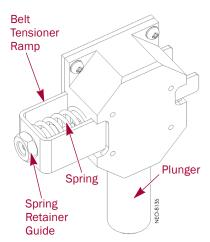
Figure 2-6: Top Pulley Spring Tensioner
