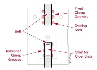
Figure 3-14: Attaching the New Belt to the Tensioner Clamp
