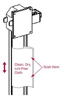
Figure 3-23: Wiping the BDA Pole with Clean, Dry, Lint-Free Cloth
