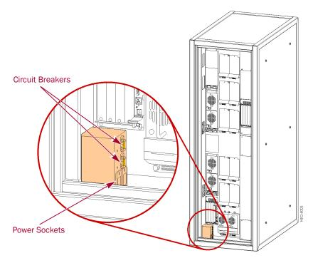
Figure 1-3: Circuit Breaker and Power Cord Locations
