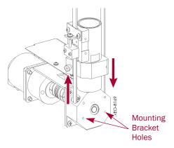
Figure 3-13: Belt Feed Through the LHA
