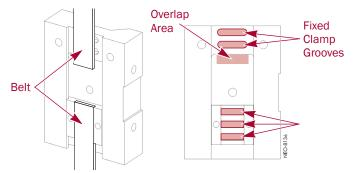
Figure 3-15: Belt Backplate Showing Clamp Grooves
