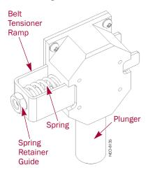
Figure 3-8: Top Pulley Spring Tensioner
