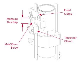
Figure 3-9: Shuttle Mount Assembly on BDA
