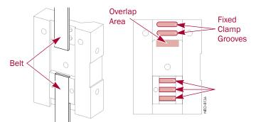
Figure 2-13: Belt Backplate Showing Clamp Grooves
