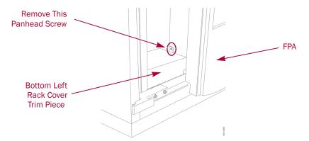
Figure 1-4: Remove the Bottom Left Rack Cover Trim
