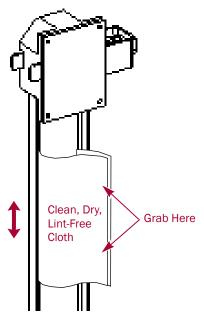
Figure 2-16: Wiping the BDA Pole with Clean, Dry, Lint-Free Cloth
