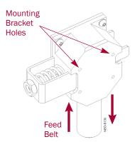
Figure 2-10: Belt Feed Through the UHA
