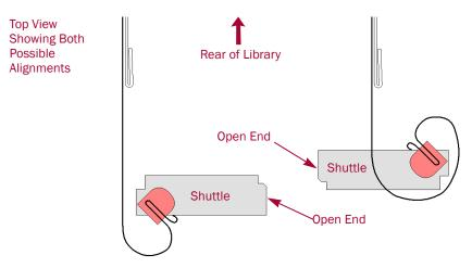
Figure 3-18: Verify Flex Cable Wrapped Correctly Around Shuttle Spooler
