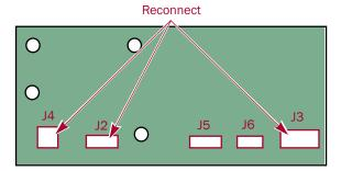
Figure 3-22: Reattach the J2, J3, and J4 Drive PWA Connectors
