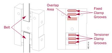
Figure 3-10: Clamp Grooves on the Backplate
