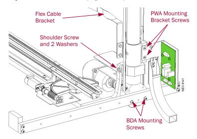
Figure 3-17: Reinstall Track Assembly to New Rear BDA
