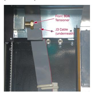
Figure 4-2: Position the J3 Cable Behind the Tensioner
