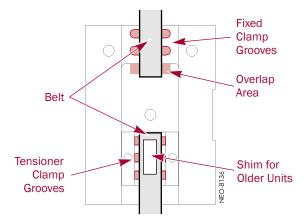
Figure 2-12: Attaching the New Belt to the Tensioner Clamp
