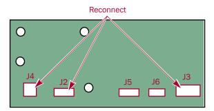
Figure 2-15: Reattach the J2, J3, and J4 Drive PWA Connectors
