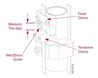
Figure 2-7: Shuttle Mount Assembly on BDA
