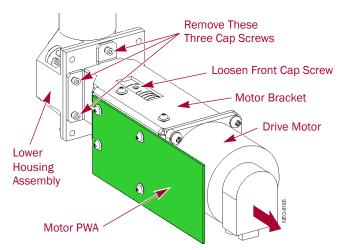
Figure 2-9: Location of the Drive Motor Screws
