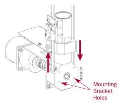
Figure 2-11: Belt Feed Through the LHA
