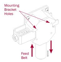
Figure 3-12: Belt Feed Through the UHA
