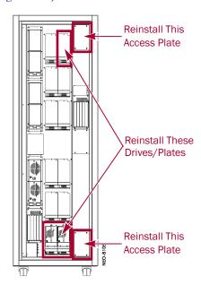
Figure 4-1: Reinstall Rear Panels or Drives
