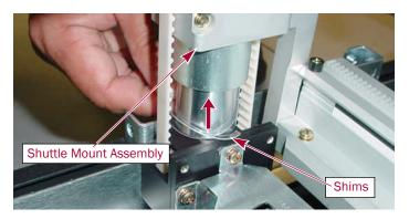
Figure 2-5: Slide Shims up the BDA
