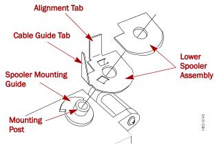
Figure 8. Shuttle Spooler Components
