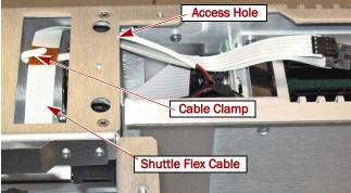
Figure 12. New Flex Cable Routed through the Access Hole
