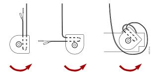
Figure 9. Wrapping the Cable Around the Spooler
