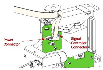
Figure 5. Front View of Shuttle Cables
