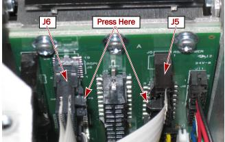
Figure 3. Press the J5 and J6 Release Latches to Release
