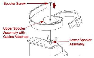
Figure 6. Removing the Upper Spooler Assembly
