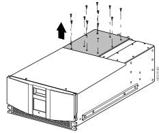
Figure 1. Remove Fan Cover Screws
