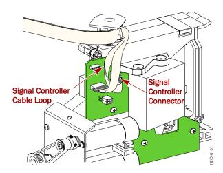
Figure 11. Connect the Shuttle Signal Controller Cable
