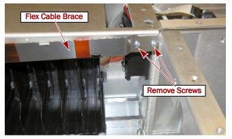
Figure 7. Location of the Flex Cable Brace Hexhead Screws
