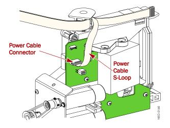
Figure 10. Connect the Shuttle Power Cable
