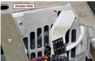
Figure 4. Access Hole Behind the Card Cage PWA
