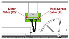
Figure 4. Cable Connections on Flex Cable Card
