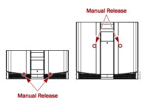
Figure 1. Manual Door Release Locations
