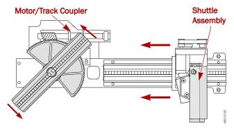
Figure 2. Top View of Shuttle Track Showing Movable Section
