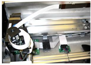
Figure 6. Flex Cable Position Around Shuttle Spooler
