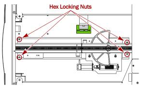
Figure 5. Remove Hex Locking Nuts
