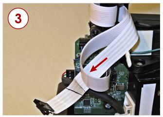
Figure 19. Insert Power Cable Through Signal Cable Loop
