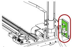
Figure 4. Rotary SPI Board Location (Rear View)
