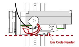
Figure 16. Flex Cable Must NOT Extend Beyond Reader
