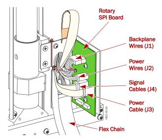
Figure 5. Rotary SPI Board in Rear Z-Axis Assembly (Rear View)
