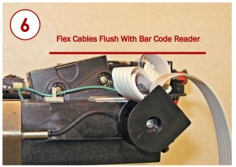
Figure 22. Cables Flush with Bar Code Reader
