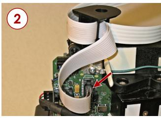
Figure 18. Loop & Insert Signal Controller Cable Into J4
