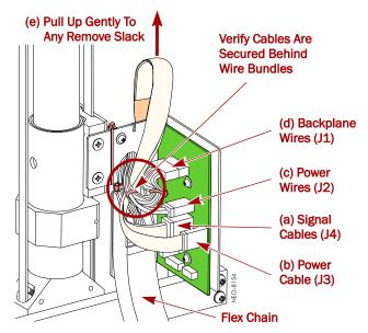
Figure 10. Rotary SPI Shuttle Cable Connections
