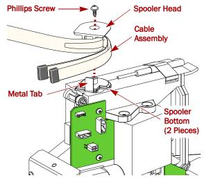
Figure 8. Removing the Cable from the Spooler Head
