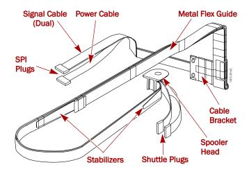
Figure 1. Shuttle Cable Assembly
