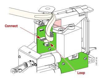
Figure 14. Connect the Power Cable
