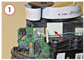
Figure 17. Secure Plastic-Coated Clamp to Shuttle
