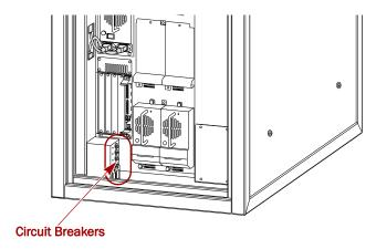
Figure 2. Location of Circuit Breakers in Rear
