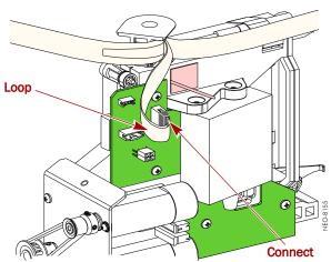
Figure 13. Connect the Signal Controller Cable
