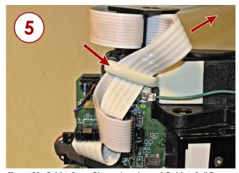
Figure 21. Fold & Press Clamp Arm Around Cables; Pull Excess
