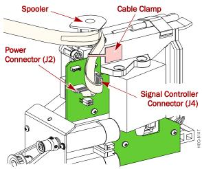
Figure 7. Shuttle PWA and Cables (Front View)
