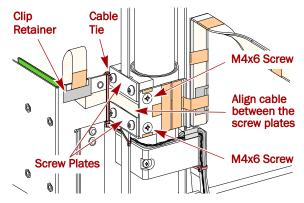
Figure 9. Attach Cable Assembly to I-Axis Bracket
