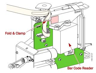
Figure 15. Connecting the Cable to the Shuttle PWA
