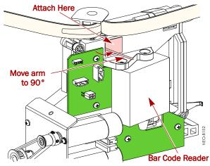
Figure 12. Attach the Clamp
