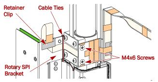
Figure 6. Key Components on Rear Z-Axis Assy. (Front View)
