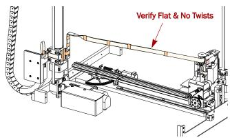
Figure 11. Final Position of Cable Assembly
