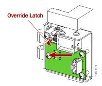
Figure 3. Media Drawer Latch Release, Rear View
