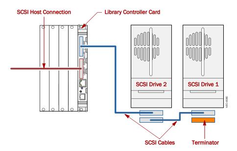
Figure 8-1: Basic SCSI Network with Two SCSI Drives
