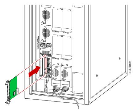
Figure C-4: Inserting the Partition Controller Card into the Library
