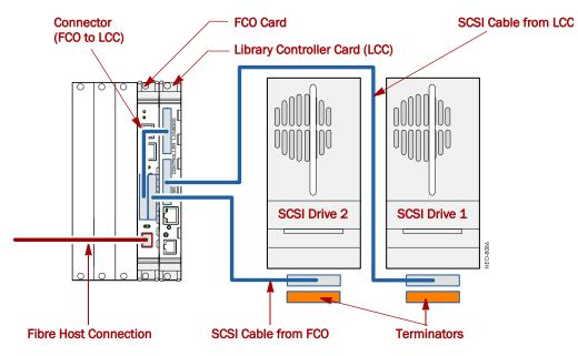
Figure 8-2: Typical Fibre Channel Network with Two SCSI Drives
