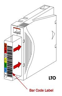
Figure 4-10: Bar Code Label Installation
