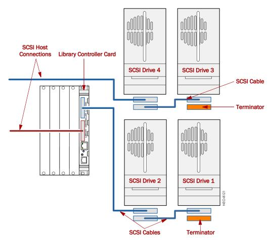
Figure 8-3: Four SCSI Drives on a Two Host SCSI Network
