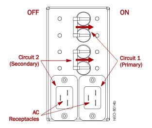
Figure 1-7: NEO 8000 Circuit Breakers Showing Primary and Secondary Circuits
