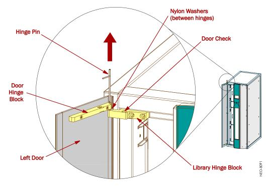
Figure 2-7: Attaching the Doors
