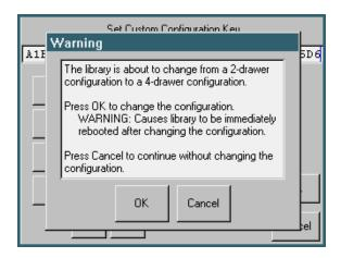
Figure 9-3: Configuration Key Warning Screen
