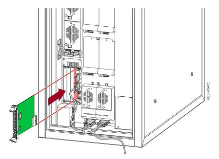
Figure C-3: Inserting the Router Card into the Library
