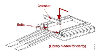
Figure B-6: Removing the Rear Crosspiece
