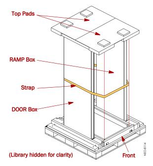
Figure 2-3: RAMP and DOOR Box Locations
