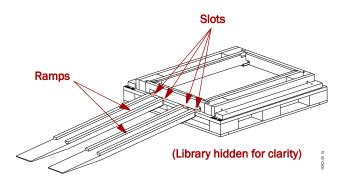
Figure 2-4: Placing the Ramps in Position
