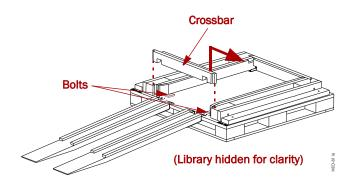
Figure 2-5: Removing the Rear Crosspiece
