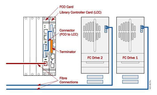
Figure 8-4: Typical Native Fibre Channel Configuration
