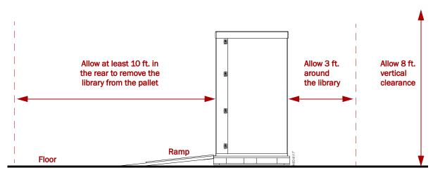
Figure 2-1. Unpacking Space Requirements
