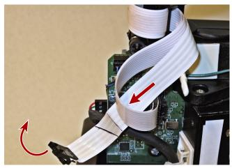
Figure 11. Insert Power Cable Through Signal Cable Loop
