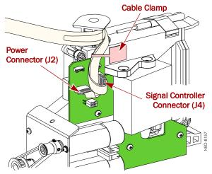
Figure 4. Shuttle PWA and Cables (Front View)
