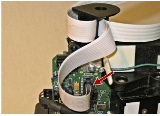
Figure 10. Connect the Signal Controller Cable
