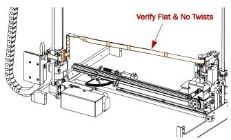
Figure 7. Final Position of Cable Assembly
