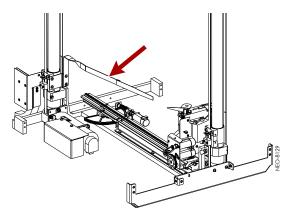
Figure 15. Metal Flex Guide Location (Cable Hidden)
