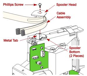
Figure 5. Removing the Cable from the Spooler Head
