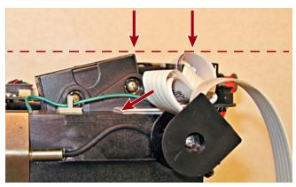
Figure 14. Flex Cable Must NOT Extend Beyond Reader
