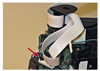
Figure 12. Connect the Power Cable
