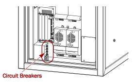
Figure 2. Location of Circuit Breakers in Rear
