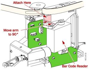
Figure 9. Attach the Clamp
