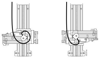
Figure 8. Wrapping the Shuttle Cable Around the Flex Cable Retainer
