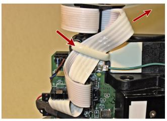
Figure 13. Connecting the Cable to the Shuttle PWA
