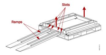
Figure B-4: Placing the Ramps in Position
