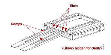
Figure 2-4: Placing the Ramps in Position
