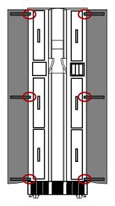
Figure 2-9: Attaching the Doors
