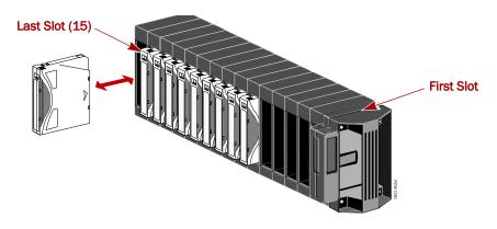
Figure 4-3: Inserting Cartridges Into a Mail Slot Magazine
