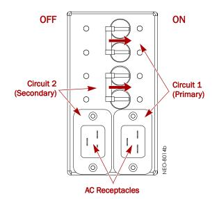
Figure 1-8: NEO 8000e Circuit Breakers Showing Primary and Secondary Circuits
