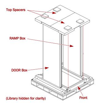
Figure 2-3: RAMP and DOOR Box Locations
