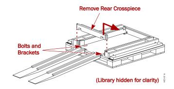
Figure 2-5: Removing the Rear Crosspiece
