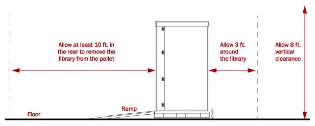
Figure 2-1. Unpacking Space Requirements
