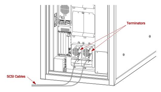
Figure 3-3: Basic SCSI Network with Two SCSI Drives
