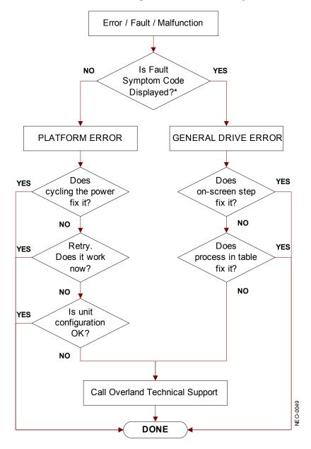
★ For a CARTRIDGE ERROR an FSC may or may not be shown. If the cartridge won't eject, normal operation is impossible. Call Overland Technical Support.
