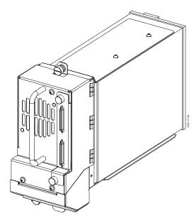
Figure 1-11: NEO 8000e SCSI Drive Assembly
