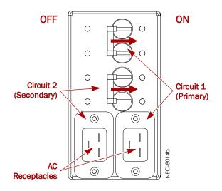
Figure 3-4: NEO 8000e Circuit Breakers (OFF Position)
