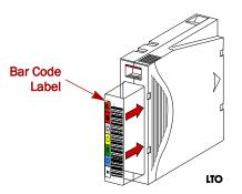
Figure 4-1: Bar Code Label Installation
