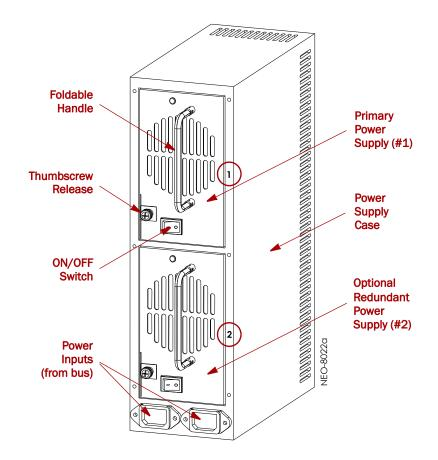
Each power supply case holds two power supplies (Figure 1-7). The upper power unit is the primary power source while the lower unit is the redundant power source.
