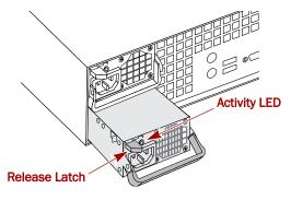
**4.** Pull the **module** out of the chassis, catching the body of the module in the other hand, and set it aside.
