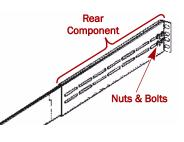
**NOTE:** For some racks, only two bolts can be used with the rear component due to the location of the slots. This does not impact the stability of the rails.
