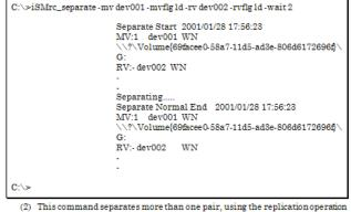
(2) This common separates more than one pair, using the representation operator file. In this example, a monitoring time interval of 2 seconds is specified with -wait.
