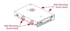
**2.** Use the **supplied screws** in the appropriate holes to secure the drive.
