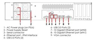
1. Connect either one or both of the 10 Gb Ethernet ports to the **network** ports of a switch, hub, or router on the same LAN as the host system being used to manage the QuikStation.
