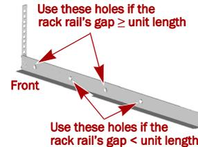
4. Align the **left-front flange** with the two marked holes on the front rack rail and loosely attach the left-side mounting rail with two screws.
