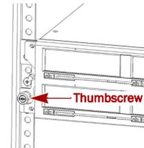
2. Using the **thumbscrews**, anchor the QuikStation 8 bracket right and left to the rack.
