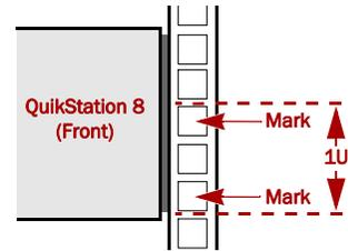
1. Determine the **2U area** where the QuikStation 8 is to be mounted and mark both sets of **first** and **third** holes of the bottom 1U on the front.
